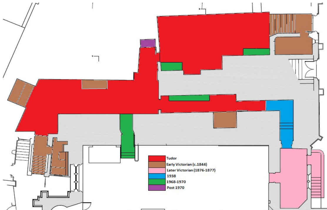
Figure 11 - Plan showing the construction of the crypt and its features by time period, from Dr George Roberts Report on the Crypt of St Peter ad Vincula December 2013.
